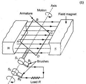
**Working** When a closed armature coil rotates in a uniform magnetic field with its axis perpendicular to the magnetic field, the magnetic flux linked with the loop changes and emf induces in the coil. Let initially angle between area vector of coil and magnetic field *B* is 0°. Thereafter, *AB* comes downward and *CD* upward then by Fleming's right hand rule induced current flows from *B* to *A*.
